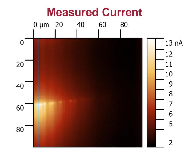
Linecuts (blue line in picture above) of measurements with different optical laser output powers were made showing that the current increase is the same for both lasers while the 488 nm laser operates at a optical power about 16 times higher than the 633 nm laser.
