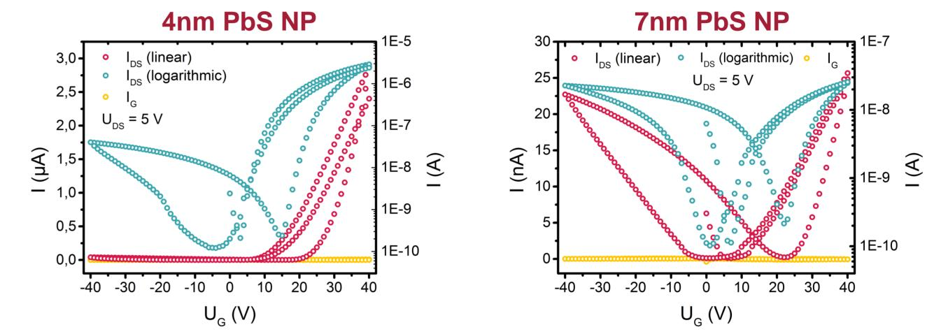
On-off modulation of about 4.5 and 2.5 orders of magnitude for e<sup>-</sup> and h<sup>+</sup> conductivity in case of the 4 nm PbS NP and 2.5 orders of magnitude for both charge carriers in
