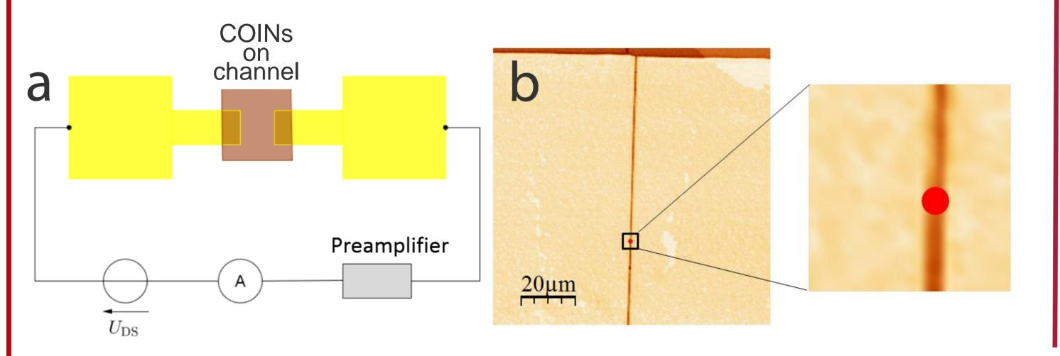
The sample is raster scanned with the laser and the current across the channel is used as contrast information. As shown in c), we measure a strong current modulation when the junction is illuminated. To verify this, we measure transport across the channel for different optical intensities and at constant bias of 3V d).
