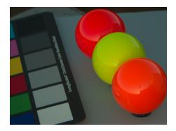
Figure 2: Spheres covered in three different multilayer paint varieties for utility vehicles ("pearl white" primer, fluorescent red/yellow/orange paint, clear coat). Note the outstanding chroma of the paints, and their luminance, which even in the non-specular part is higher than the one of the 90% white ColorChecker patch.
