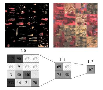
Top left: input texture map. Top right: Same map after filling Fig. 3. operation. Bottom: fill, downsampling from L0 to L2, upsampling L2 to L0. Hatched boxes mark unused texels that were filled during upsampling.
