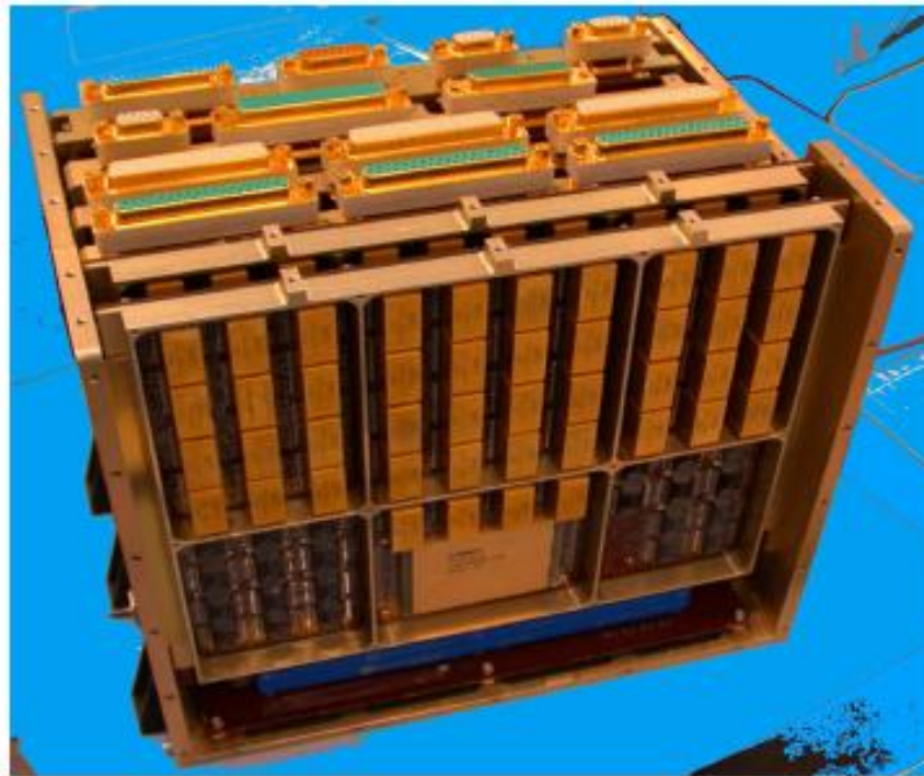
Figure 2.9: Block diagram (top) of the SCU with the main modules (see also Paragraph MDP in 2.3.3.2) and a picture (bottom) with removed panels, showing the Memory module in front (Image: courtesy of Thales Alenia Space).
