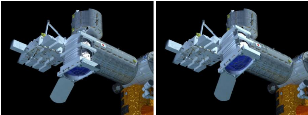
Figure 1.2: The JEM-EUSO telescope in nadir mode (left) can be tilted (right) to increase the effective area (Image: JEM-EUSO Collaboration).
