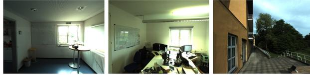
**Fig. 11.** Test scenes for multi-camera rig evaluation: corridor (left) exhibits few gradients, repetitive ceiling texture and glossy highlights; office (center) shows many trackable gradients; veranda (right) is an outdoor scene with large depth variations.
