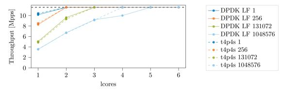
Replace double-buffering mechanism (t4p4s) through lock-free DPDK hash table implementation (DPDK LF)
