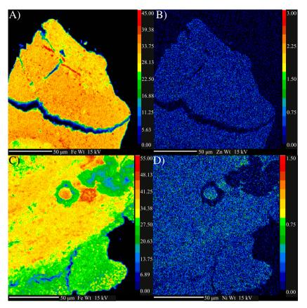
**Fig. 4.** Electron microprobe maps showing the distribution and weight percent for (A) Fe and (B) Zn in sample ZnBF2, and (C) Fe and (D) Ni in sample NiBF2. Color bars indicate the weight percent ( $\pm 1\%$ ) of the corresponding element. (For interpretation of the references to color in this figure legend, the reader is referred to the web version of this article.)
