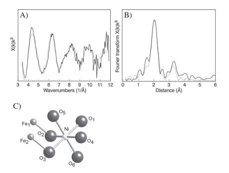
**Fig. 1.** (A) EXAFS and (B) Fourier transform of the EXAFS for Ni sorbed to ferrihydrite. Solid lines are data; dotted lines are fit. (C) Molecular cluster used to fit the EXAFS data, where  $O_1-O_6$  = octahedral oxygen atoms in Ni first shell coordination sphere and  $Fe_1-Fe_2$  = iron in ferrihydrite Fe octahedra.
