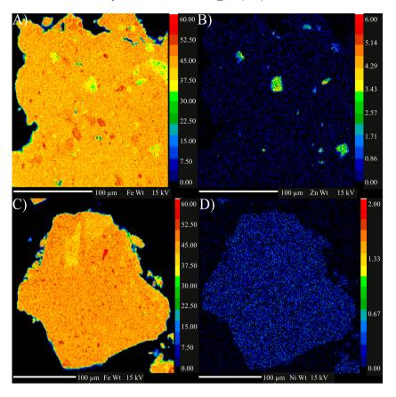
**Fig. 3.** Electron microprobe maps showing the distribution and weight percent for (A) Fe and (B) Zn in sample ZnFh-2, and (C) Fe and (D) Ni in sample NiFh-2. Color bars indicate the weight percent ( $\pm 1\%$ ) of the corresponding element. (For interpretation of the references to color in this figure legend, the reader is referred to the web version of this article.)
