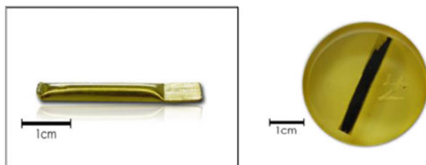
Fig. 1 The image on the left shows a gold capsule after it had been filled with a ferrihydrite-glucose mixture under anoxic conditions in a glovebox and welded shut. These gold capsules were then incubated at a temperature of 170 °C and a pressure of 1.2 kbar for 1–100 days. The image on the right shows a capsule after incubation that was embedded in resin, cut in half, and polished for microscopy investigations
