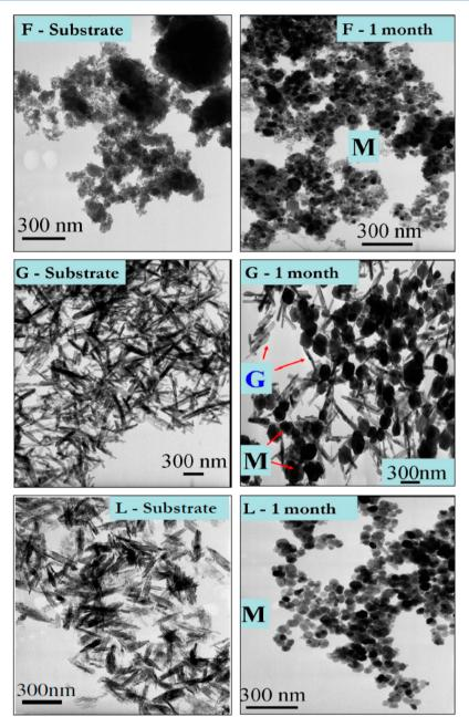
**Figure 8.** Bright field transmission electron microscopy images showing initial ferric (oxyhydr)oxides (ferrihydrite-F, lepidocrocite-L, and goethite-G) and their transformation products after their reaction with suitable amounts of Fe(II) and OH<sup>-</sup> to form stoichiometric magnetite (M). Transformation product of G indicates the presence of M and untransformed G. Reproduced with permission from ref 37. Copyright 2012 Elsevier.
