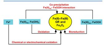
Figure 5. Overview of different pathways for the formation of magnetite  $(Fe_3O_4)$  and green rust (GR).
