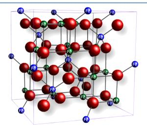
**Figure 1.** Ball and stick model of the unit cell of magnetite. Octahedral Fe ions are in green, tetrahedral Fe ions are in blue, oxygen ions are in red. Created using CrystalMaker for Windows version 2.2.
