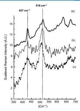
**Figure 15.** Microprobe Raman spectra of different green rusts (GRs): (a) natural GR, (b) synthetic  $GR(CO_3^{2-})$ , and (c) correspond to synthetic  $GR(Cl^-)$ . Reproduced with permission from ref 85. Copyright 1997 Elsevier.
