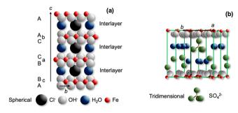
**Figure 2.** General view of the crystal structure of green rusts: (a) GR-I (Cl $^-$ ) and (b) GR-II (SO $_4^{2-}$ ). Image (a) is adapted with permission from ref 26. Copyright 1998 Elsevier. Image (b) is adapted with permission from ref 24. Copyright 2003 Elsevier Masson SAS.
