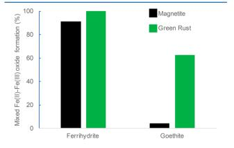
**Figure 7.** Transformation extent of ferrihydrite and goethite into mixed-valent iron minerals (magnetite and green rust) measured by Mössbauer Spectroscopy. Ferrihydrite and goethite were reacted with stoichiometric amounts of soluble Fe(II) and NaOH to form magnetite and green rust according to the reactions 3 and 4. Figure prepared by using the data reported in Table 2 of ref 51.
