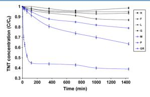
Figure 22. Fenton-like oxidation of TNT (0.11 mM) in the presence of six different iron minerals (2 g  $L^{-1}$ ) at pH 7: ( $\blacksquare$ ) hematite, ( $\blacktriangle$ ) ferrihydrite, (\*) lepidocrocite, ( $\spadesuit$ ) goethite, ( $\bigcirc$ ) magnetite, ( $\triangle$ ) pyrite, ( $\diamondsuit$ ) green rust.  $H_2O_2$  (3%, w/v). Reproduced with permission from ref 512. Copyright 2008 Elsevier.
