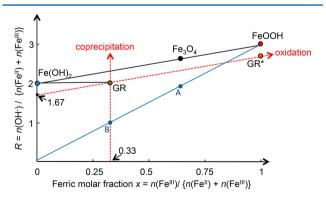
**Figure 6.** Mass-balance diagram representing the synthesis of magnetite ( $Fe_3O_4$ ) and green rust via coprecipitation and oxidation. GR correspond to green rust and GR\* to the fully oxidized form of GR (i.e., Mössbauerite). Point A corresponds to the mixture [2/3 FeOOH, 1/3 Fe(II)] and point B is mixture [1/3 FeOOH, 2/3 Fe(II)]. Adapted with permission from ref 31. Copyright 2006 Elsevier Masson SAS.
