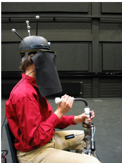
Figure 1: A participant equipped with tracking helmet, hmd and cover using the pointing device to point towards previously learned locations.
