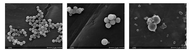
Figure 2. SEM pictures of the synthesised microspheres. From left to right: calcinated cores particles in anatase  $cTiO_2$ ; cores after porous amorphous  $aTiO_2$  coating;  $cTiO_2@aTiO_2$  core@shell after  $SiO_2$  coating and calcination
