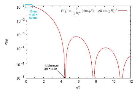
Figure 10: Form factor for a large spherical particle.
