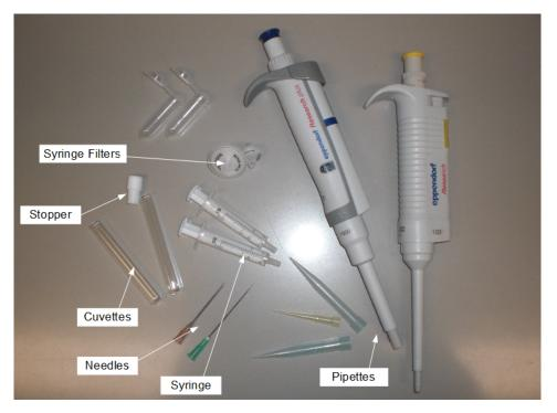
Figure 16: Some important equipment for preparation.
