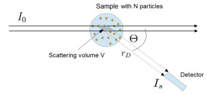
Figure 5: Schematic construction of a light scattering apparatus.
