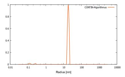
Figure 21: In the editor stored CONTIN-data plotted with Gnuplot. In this example you find particles with a radius of  $R \approx 15$  nm.
