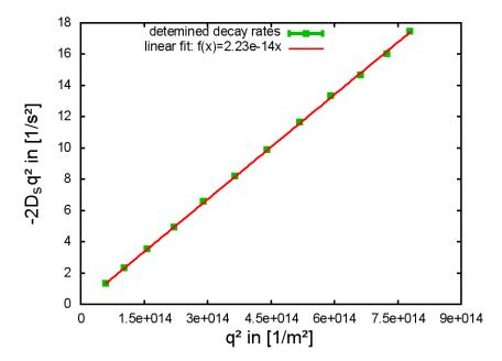
**Figure 24:** Example plot of  $\Gamma$  vs.  $q^2$  and a linear fitting. From the slope one obtains the diffusion coefficient  $D_{\rm s}$ .
