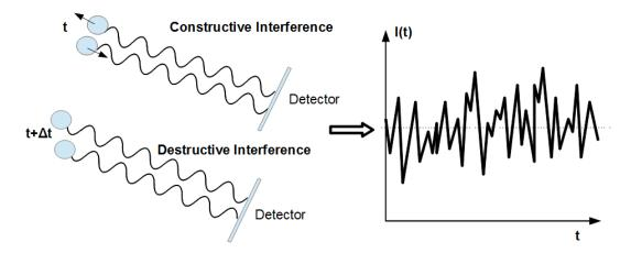
Figure 12: Illustration of how the time-dependent interference can occur. The resulting scattering intensity fluctuates around the average  $\langle I \rangle$ , which is used for SLS.
