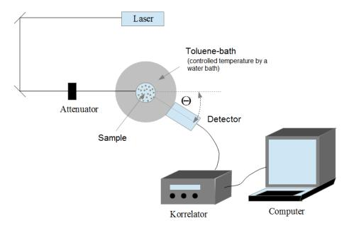
Figure 14: Schematic structure of a light scattering apparatus.
