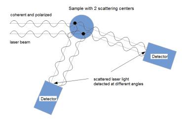
Figure 7: Schematic representation of light scattering from two scattering centers in a large particle. Depending on the scattering angle at which the intensity is detected, different interferences of the scattered radiation occur.
