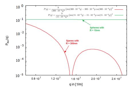
Figure 11: Form factors of spheres with different sizes, P(q) as functions of q.
