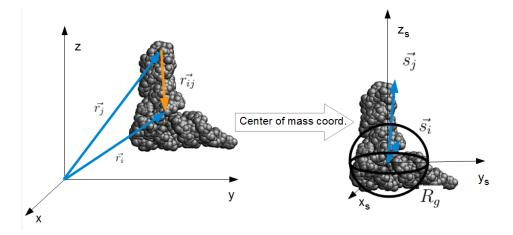
Figure 8: Transformation to center of mass coordinates.
