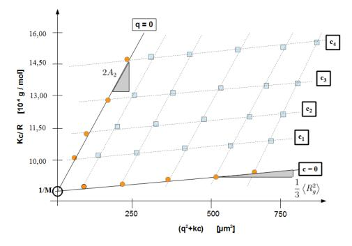
**Figure 9:** The Zimm plot is obtained by plotting of Kc/R over  $q^2 + kc$  (small squares represent the measured values). By extrapolation of  $q^2$  to zero and c to zero (points are the extrapolated values)  $R_{\rm g}$  and  $A_2$  can be determined from the corresponding slope and by the y-intercept we get the molar mass M.
