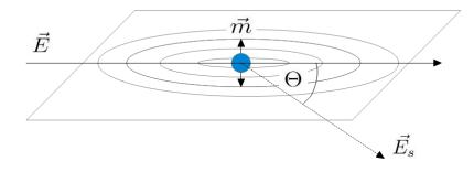
Figure 2: Induction of an oscillating dipole caused by an incoming electromagnetic wave
