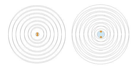
Figure 4: Interference pattern of light scattered from small particles (left) and from larger particles (right) illustrated with two scattering centers.
