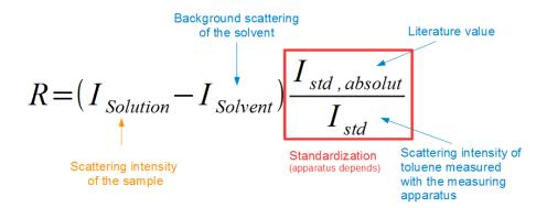
Figure 6: Measured Rayleigh ratio.
