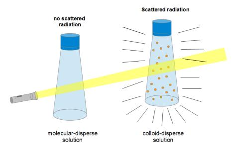
Figure 1: Schematic representation of the Tyndall effect.
