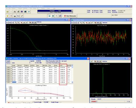
Figure 20: Screenshot during the measurement. Intensity fluctuations (top right), particle size (bottom right) determined by the CONTIN-algorithm that uses the values of the correlation (top left). The measured  $\frac{Kc}{R}$ -values at each angle are shown in the table and are used for the SLS evaluation.
