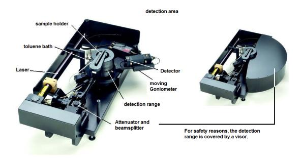
Figure 15: Setup of the 'ALV/CGS-3 Compact Goniometer System'.
