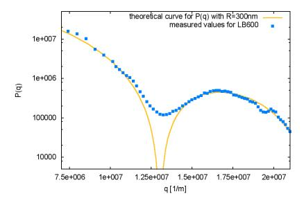
Figure 22: Example plot of the form factor of LB600 with experimentally determined intensity (solid circles) and the theoretical model for monodisperse spheres (solid line). In this example the particles have a radius of  $R \approx 300$  nm.
