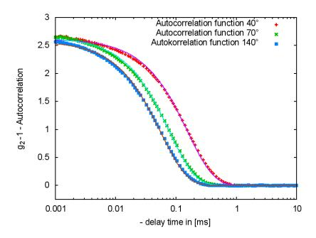
Figure 23: Example plots of the intensity-time autocorrelation function  $g_2(\tau) - 1$  with data fitting using Eq. 39.
