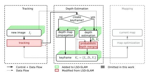
Fig. 3. Overview over the LSD-SLAM algorithm and our extensions.
