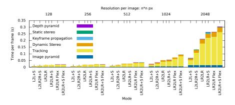
Fig. 10. Timing evaluation. The L2L+S configuration which works best for stereo rigs runs at more than 15 fps even for 4 Megapixel images. There is just small computational overhead introduced by static stereo and nonrigid tracking. Note that there is some overhead for CPU/GPU synchronization which consumes significant time for smaller resolutions. Also note that the three tasks at the top that are only performed when the keyframe is updated have a very small average per frame contribution.
