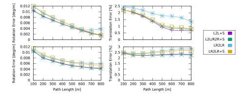
Fig. 7. Results from the KITTI odometry benchmark scenes 06 (top) and 08 (bottom). Note that static stereo seems to improve quality significantly. Tracking and depth estimation between different cameras from different frames produces worse results in the scenes because of errors that are introduced by more occlusions on longer baselines.
