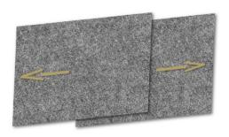
al. 1993) Generally, these methods are based on the idea that the cross-correlation of the image and a shortly afterwards taken image is calculated for small displacements: the best fitting displacement accounts for the movement.
