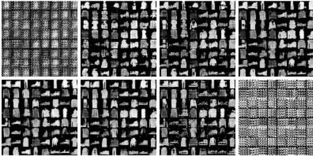
Figure 4.8: The fmnist_dcgan , using the MOMENTUM optimizer. The top row shows the images generated at epoch 2, 4, 6, and 8. In the second row, epochs 10, 12, 13, and 14, are presented, from left to right. With a value of 0.5 for the momentum term, the model learns to match the distribution of the training data but collapses after the fourteenth epoch.
