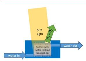
Figure 1a: Overall design of our system for plasmonic solar hydrogen production via photon driven H<sub>2</sub>O splitting.
