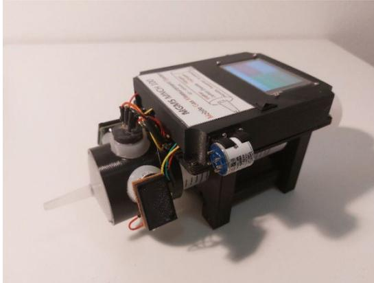
**Figure 3:** A first prototype of the gas measurement system with three sensors, a device for data logging with a display, a power supply, a rotary potentiometer and a main switch.
