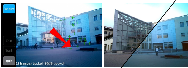
Figure 7: Rephotography. A Frankencamera platform lets us experiment with novel capture interfaces directly on the camera. Left: The rephotography application directs the user towards the location from which a reference photograph was taken (by displaying a red arrow on the viewfinder). Right: The reference photograph (above and left), which was taken during the morning, overlaid on the image captured by the rephotography application several days later at dusk.
