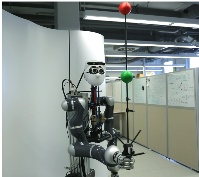
Fig. 1. Robot Apollo balancing an inverted pole. This experimental platform is used as a demonstrator of the automatic tuning framework.
