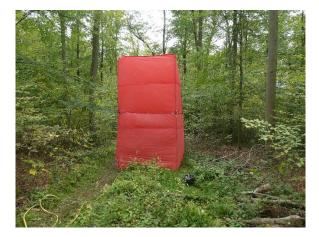
A rain simulator was used in Schönbuch nature park to measure how soil erodes in skid trails.
