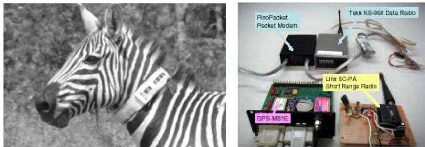
Figure 26: Plains Zebra wearing a ZebraNet collar (left) [SaSa04], corresponding hardware of a tracking collar [JOWM + 02]
