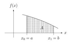
Solution: cut the area in rectangles and let the number of rectangles in the area  $a=x_0< x_1<\ldots< x_n=b$  go to infinity  $(n\to\infty)$ :
