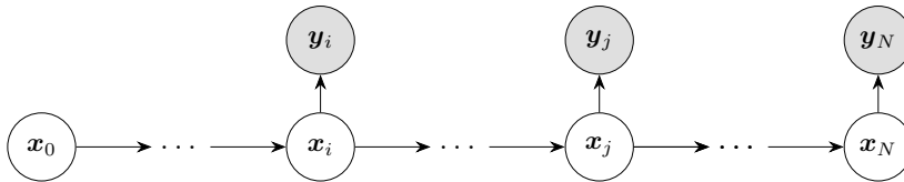
Figure 2.3: Graphical model of the described probabilistic state-space model. The Markov property can be read off from the chain-structure in \mathbf{x}_{0:N} .
