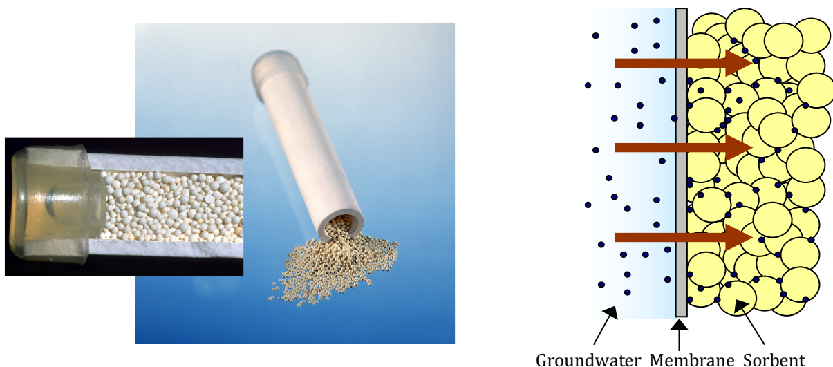
Fig. 5.1: Design of a ceramic passive sampler “dosimeter” (Bopp et al., 2004; Weiß et al., 2007)
