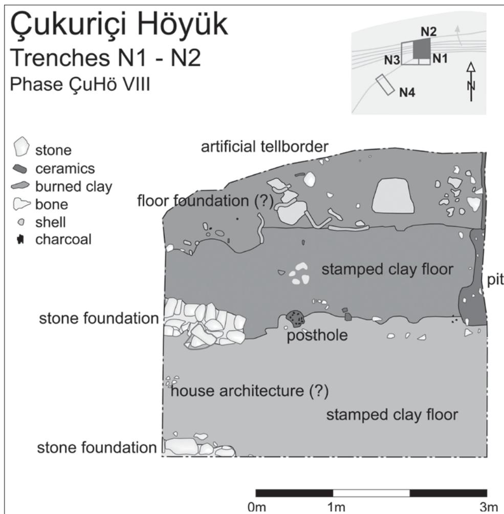
Fig. 4 Deposits of settlement phase ÇuHö VIII: architectural remains and different using horizons. Drawing by A. Buhlke, B. Horejs, A. Nordmeyer.
