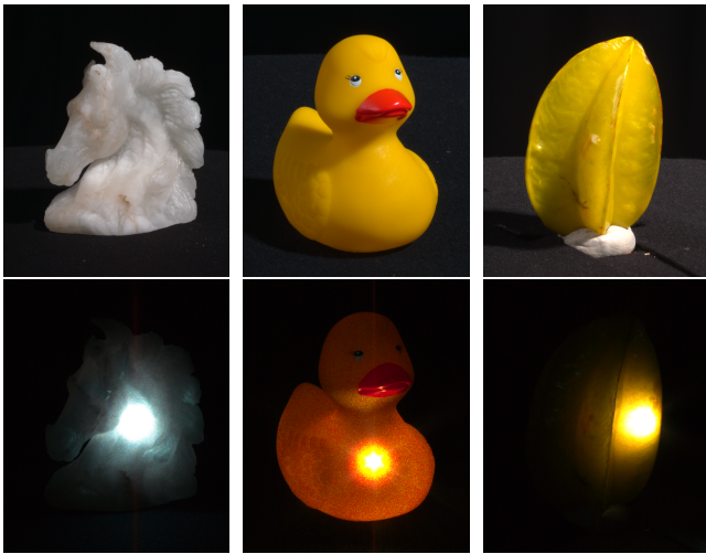
Figure 9: The test objects under indoor illumination (top row) and illuminated by all three lasers (bottom row).
