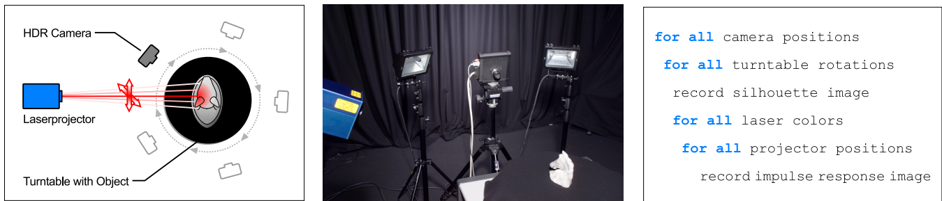
Figure 3: Acquisition setup and acquisition order. Left and middle: The laser projector illuminates the target object (resting on the turntable). The scene is observed by the HDR video camera from several positions. The two spotlights visible on both sides of the camera in the right image are used to illuminate the object during silhouette detection. Right: Acquisition order in pseudo code.
