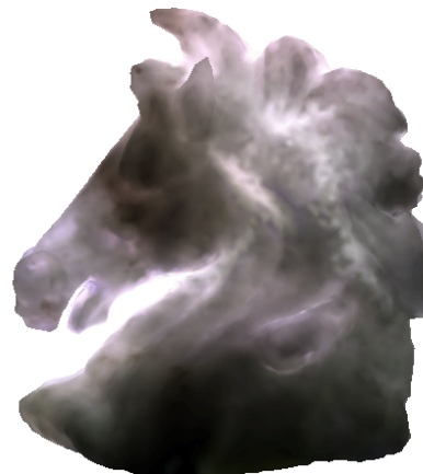
Figure 1: A model of an alabaster horse sculpture acquired by our DISCO method. Differences in material are clearly visible when the model is lit from behind. Figure 2 shows a photograph of the sculpture and Section 9 discusses the result in detail.
