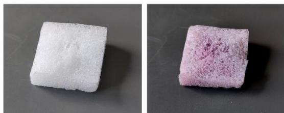
**Figure 1b:** Two steps of the preparation leading to our plasmonic water splitting system. Left: uncoated PDMS sponge. Right: PDMS sponge spiked with  $TiO_2$  and Au particles. The plasmonic nature of the Au nanostructures leads to the visible colour change of the scaffold. (corresponding to Fig. 2f).
