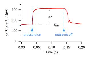
This figure shows a schematic representation of our measurement principle. When the pressure is switched on, the tissue below the nozzle is deformed and the measured ionic current (I) increases. When the pressure is switched off again, the tissue relaxes and the current decreases. From a combination of the minimum ( $I_{\min}$ ) and maximum ( $I_{\min}+\Delta I$ ) currents, the elasticity of the sample can be deduced. Typical currents are in the microampere range.
