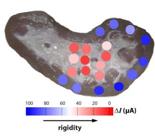
Comparative measurements of elasticity in different parts of a sectioned pig's kidney using our new device. The difference in electric current  $\Delta I$ , measured when the water jet of the device is on or off, depends on the sample's elasticity. As can be seen, the inner parts of the organ are much more rigid than the margins.
