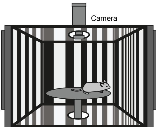
The „virtual optokinetic drum“, which has been developed by neuroscientist Thomas Münch and his group, allows faster and more objective testing of visual performance of mice than previous setups.
