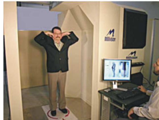
Simulating outdoor condition by a cooled wall (Millivision)
