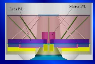
The Optics Spacecraft concept is based on XEUS heritage. It consists of a thrust cone, four equipment radius, four stiffening radius, eight sets of reinforcement rods and an external cylindrically drum.
