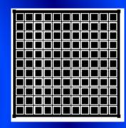
❖ The coplanar-grid technique consists of a detector anode equipped with a pair of interleaved grid electrodes and a full area electrode on the cathode side. 3D spatial resolution can be achieved with 2D coplanar anode strucure
