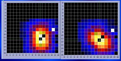
The improvement in the PSF size with new bent crystal in Laue Lens construction require a more fine spatial resolution of the focal plane increasing its polarimetric expected performance:
