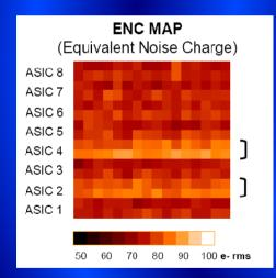
The IDEFIX ASIC: a Low noise readout 16 channels electronics: average r.m.s. 80 e
