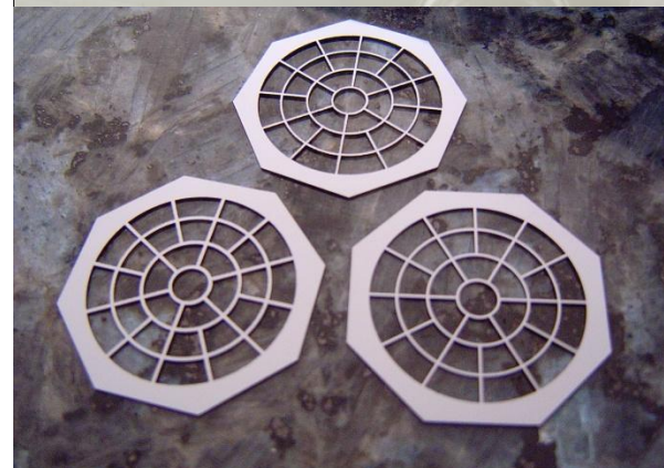
'spider web' collimator for split event suppression
