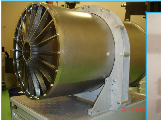
Mechanical structure: 2 spiders with 20 spokes
