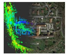
To make the SLAM system suitable for application scenarios with long-term deployment in large-scale environments, lightweight map representations should be used. Additionally, these maps should be split up into smaller map tiles, as already introduced through an approach which is called Hybrid Metric-Topological 3D Mapping.
