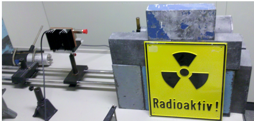
Figure 1: Experimental setup: On the left side the detector and on the right side the source. The different absorbers are put in between detector and source.
