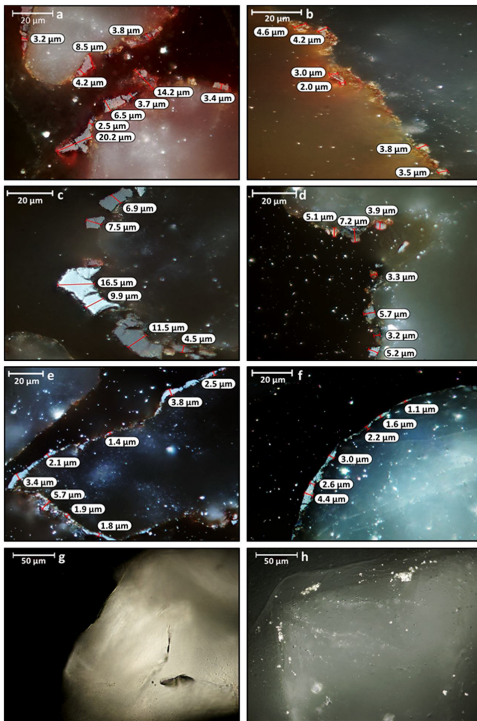
Fig. 2. Light micrographs of thin sections prepared for a) ferrihydrite coated fine sand (FH-Fine), b) ferrihydrite coated coarse sand (FH-Coarse), c) biogenic magnetite coated fine sand (Bio-Fine), d) biogenic magnetite coated coarse sand (Bio-Coarse), e) abiogenic magnetite coated fine sand (Abio-Fine), f) abiogenic magnetite coated coarse sand (Abio-Coarse), g) Pure-Fine sand and h) Pure-Coarse sand. Red bars indicate layer thickness measurements.
