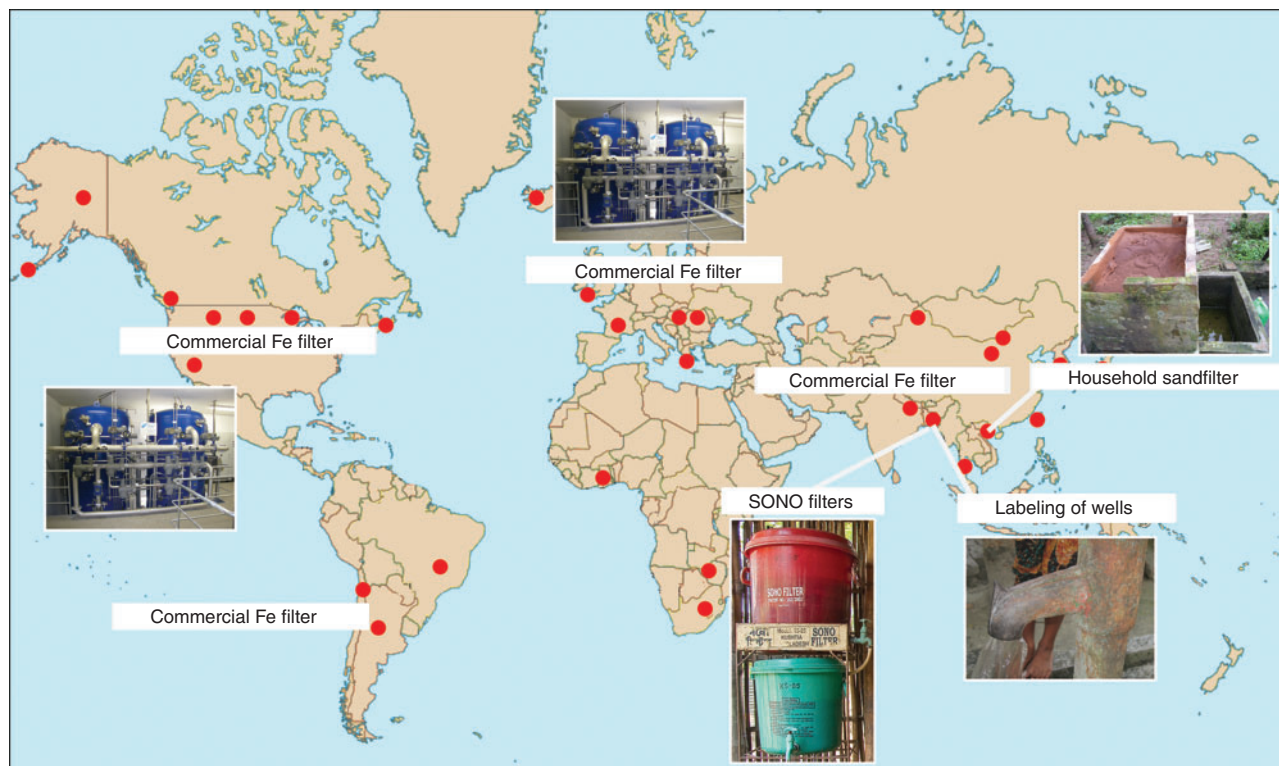
Fig. 4. Arsenic-bearing areas worldwide (red dots) and the respective main technology used in these regions to provide drinking water with As concentrations below 10 \mu\text{g L}^{-1} .
