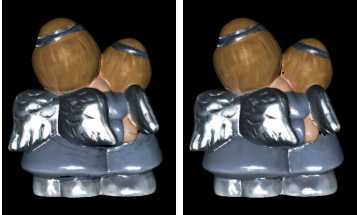
Figure 5: Left: Dark stripes on the dress and on the hand are due to depth discontinuities. Right: By discarding samples at depth discontinuities and shadow boundaries these effects have been removed.
