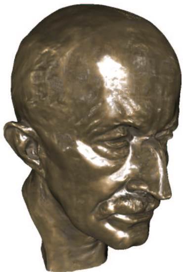
Fig. 5. A bronze bust rendered with a spatially varying BRDF, which was acquired with our reconstruction method.
