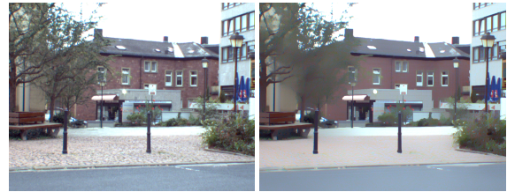
Figure 3: Left: Input Image; Right: The bilateral filter decomposition removes the details from the image and preserves sharp edges
