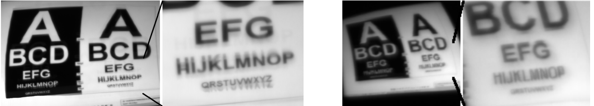
Figure 4. Our results: Reflections in a tea pot from a distance of 10 meters (left) and 30 meters (right), respectively, using the 235 mm Schmidt-Cassegrain telescope and an astronomic camera.
