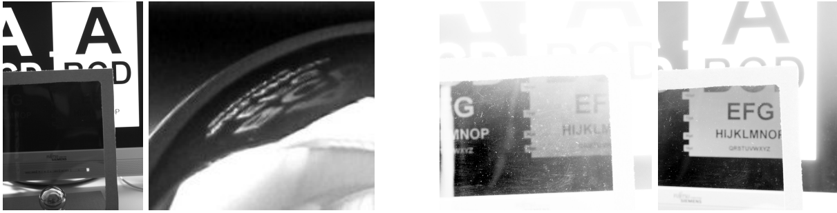
Figure 14. These images show that the protection offered by suitably aligned polarization filters is far from being perfect. While blocking most light (first image), metallic objects change polarization of light, making the monitor content readable (second image, magnification from first image). Increased exposure times still reveal the monitor contents (third image), in particular if the alignment of the two polarization filters is not perfect (fourth image).
