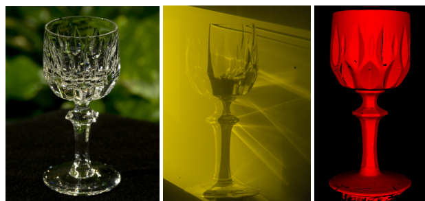
Figure 1: Fluorescent Immersion Range Scanning allows us to capture the 3D surface of challenging materials such as this crystal goblet. The object is placed into a tank filled with a fluorescent liquid which renders an incident light sheet visible. Inside the object, however, no fluorescence takes place. The surface contour is detected at the line where the intensity drops.
