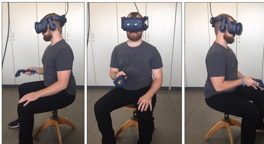
Figure 9: Photograph of the seating set-up for each participant: Participants were seated on a swivel chair while wearing the VR headset and holding the VR controller in their right hand. Rotation in the VR world was possible via self-rotation of the participant on the swivel chair, as shown. Locomotion in the VR world was possible by pulling the trigger of the VR controller. (Consent for taking and using the images was obtained.)
