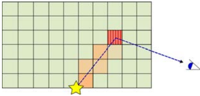
Figure 10: 2D Precomputation of the light reaching a voxel (striped texel) from the central star within the map instead of computing it for the full volume. All dust density values on the line from the central star to the texel are accumulated.
