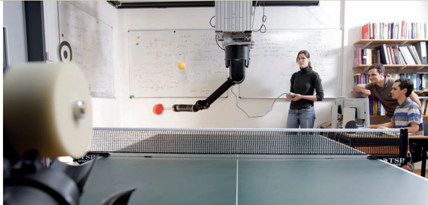
After only a short training session, this robot arm develops its own movements for playing table tennis.
