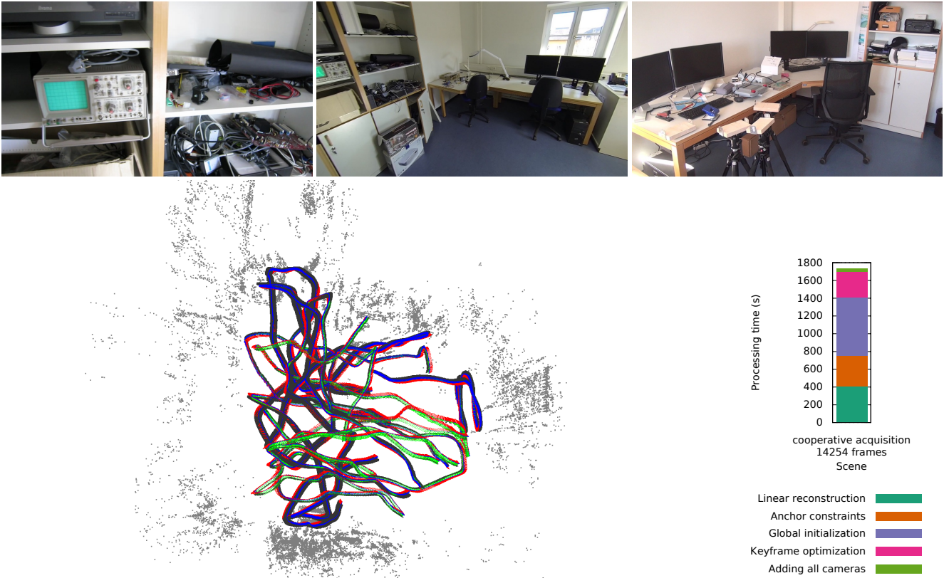
Figure 12. Example images, reconstruction visualization and timings from cooperatively captured video sequence set containing 14254 frames from three different cameras. Examples images from left to right: Canon S100, GoPro Hero3, Sony camcorder. All reconstructed camera trajectories are linked into a common global context by the anchor constraints.
