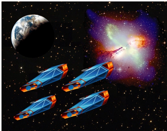
Figure 3.2: An artist's impression of original Con-X mission, which was planned to be a multi-satellite mission at first, but was redesigned into a single satellite mission. Here, four Con-X satellites are shown in formation flight, aiming at the same source to make use of their combined larger effective area. GSFC/NASA
