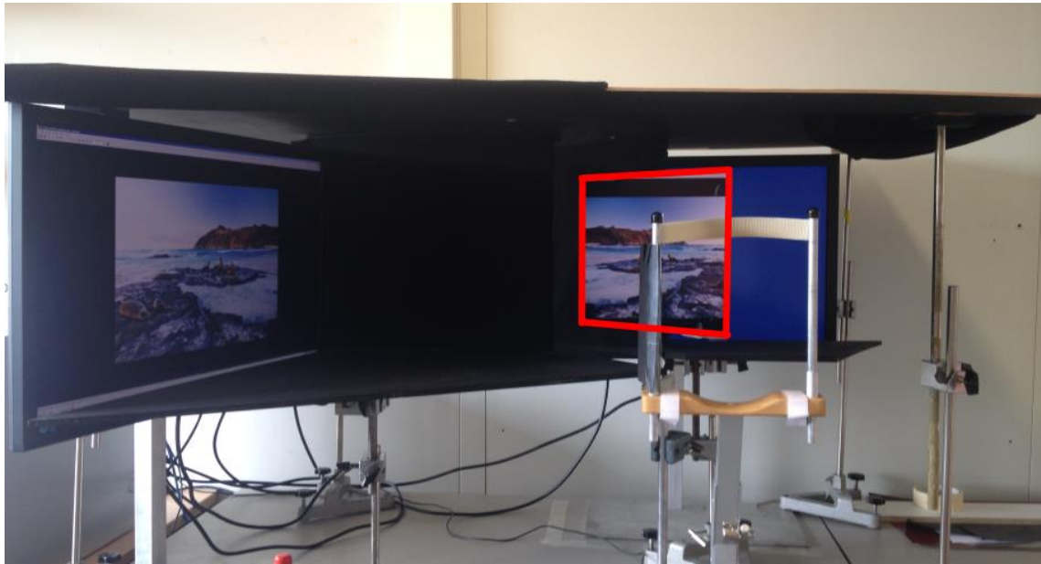
Figure 4: Set-up of the stereoscope. The mirror is indicated by the red frame.
