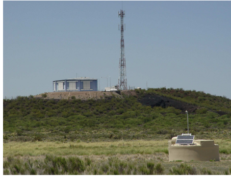
Figure 2.18: View of fluorescence observatory (back) and particle detector (front) in Auger detector [86]
