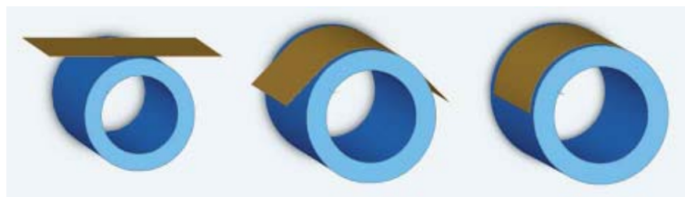
Figure 5.3: Forming an SGO sheet. When heated up to a temperature of about 600°C the glass sheet softens and wraps itself around the mold (Barcons et al., 2011).
