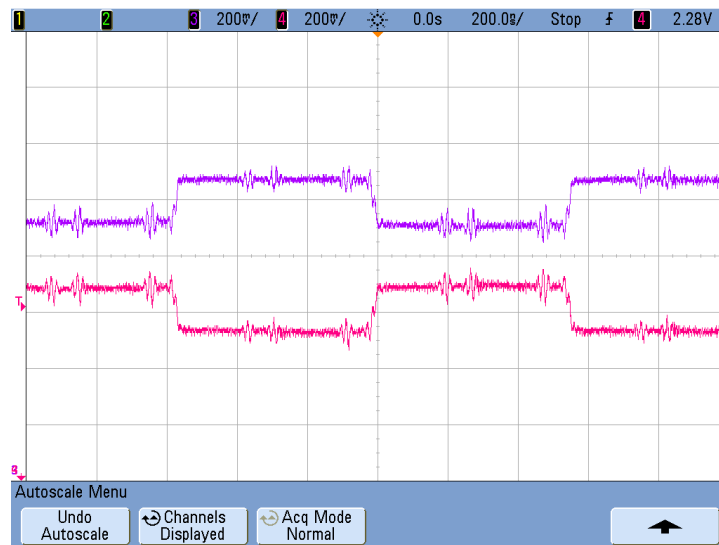
Figure 6.17: After the CAMEX signal has passed the amplification stage, there is nearly no degradation concerning noise. The offset of the differential signal can easily be adjusted at an adjustable resistor at the ADC-board. The signal has an offset common mode of \sim 2.46 V, given by the ADC.
